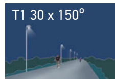
Application: Asymmetric light distribution for Narrow road.
