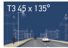
Application: Asymmetric light distribution for Urban road.
